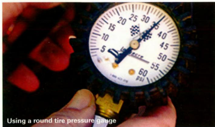
Using a round tire pressure gauge
