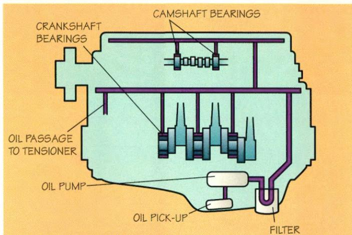
**Lubrication system components**
