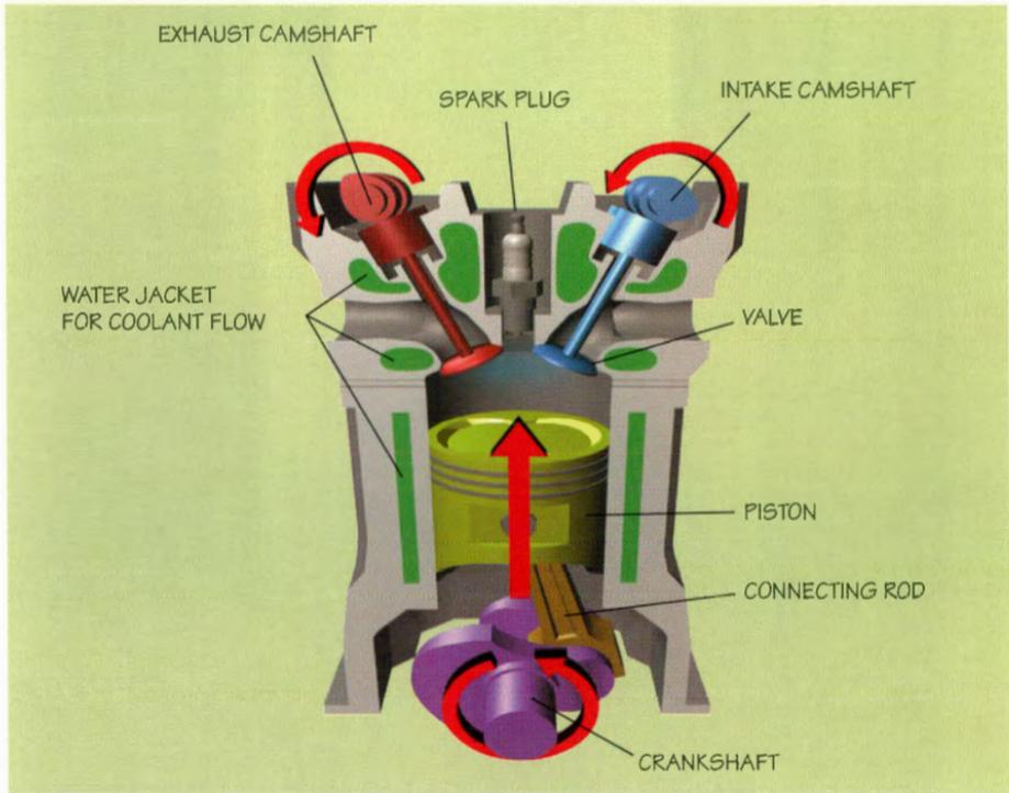
Combustion chamber components
