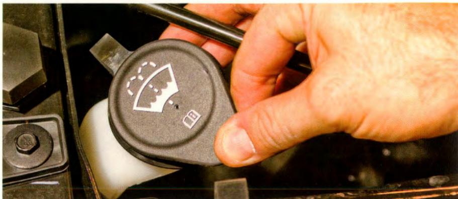
Windshield-washer fluid goes in a reservoir beneath a cap displaying a windshield wiper icon. The fluid includes detergent to clean the windshield and antifreeze to keep it from freezing in cold weather.
